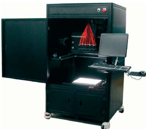
Multipoint display test station prototype Image: courtesy by Izuzu Optics, Taiwan
