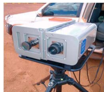
Dual VNIR and SWIR camera setup on a rotary scanner
