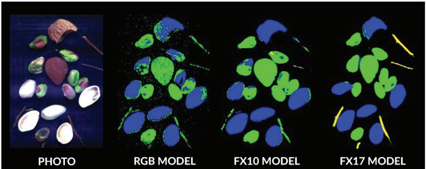
Figure 2: Photo and model predictions based on RGB camera, FX10 and FX17 data.
