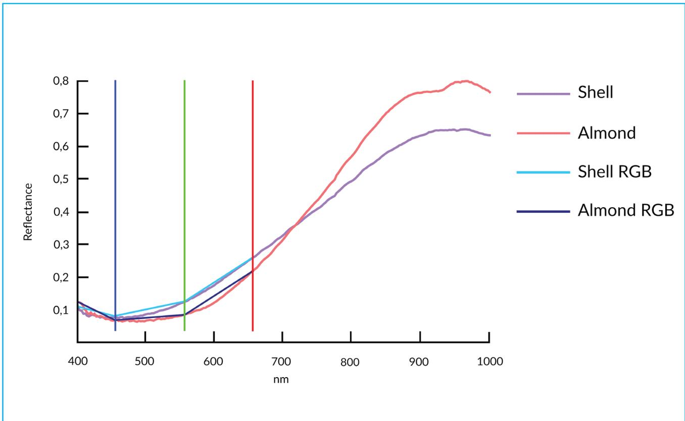
Figure 1: VNIR spectrum of an almond (FX10; Red) and shell (FX10; Magenta). RGB components of almond (dark blue) and shell (cyan). Measurable RGB camera bands are represented by respective vertical lines.
