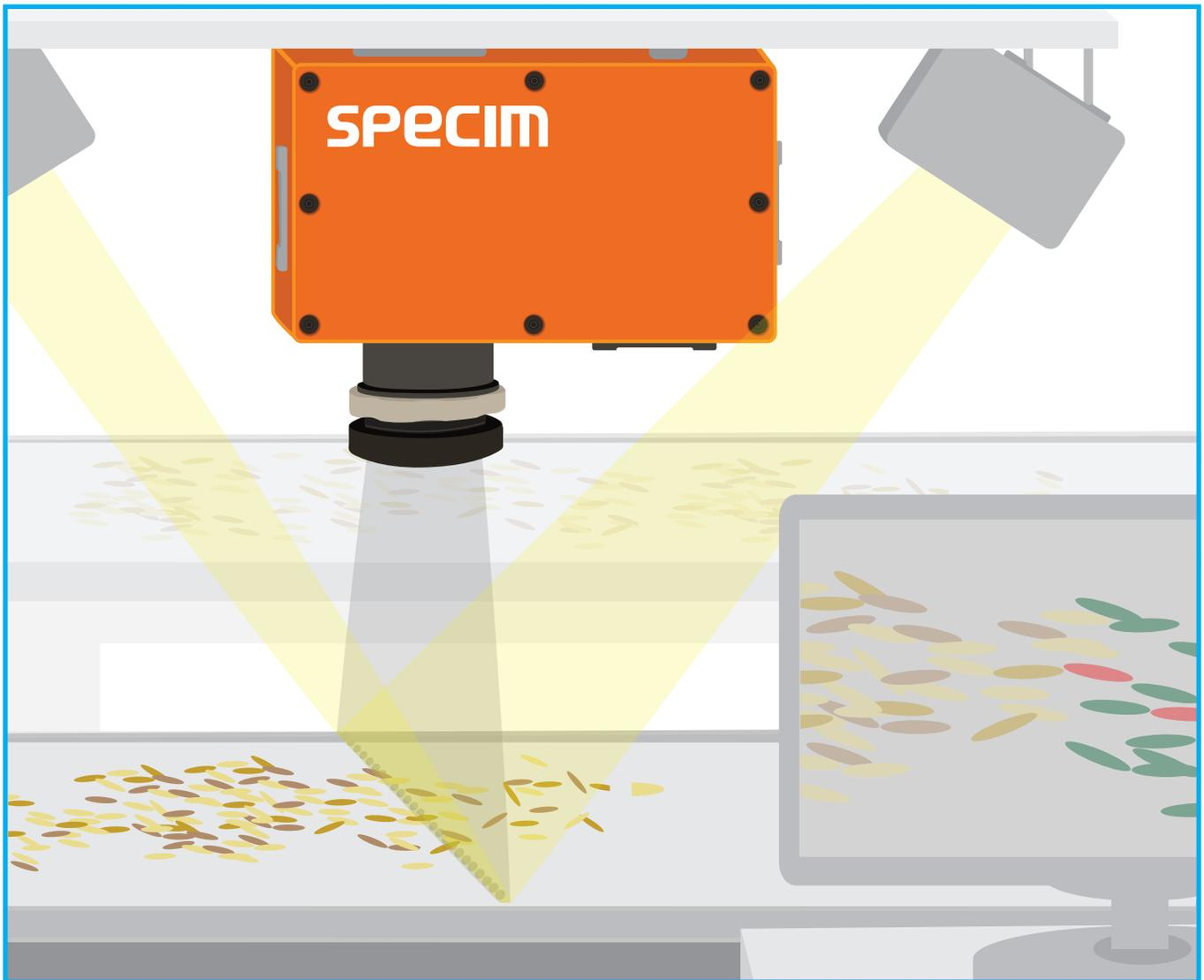
Hyperspectral cameras used in industrial environments or onboard airborne platforms (UAV or airplanes) often operate in a pushbroom fashion. Those cameras, like Specim ones, all build following the same approach:
